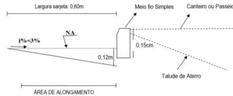
$$d = 36 \times 10^4 \times \frac{A \times R^{2/3} \times I^{1/2}}{C \times i \times L \times n}$$
